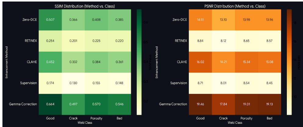
Fig 6. Heatmap: Distribution of SSIM and PSNR values across enhancement methods and weld classes.
